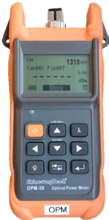
Optical Power Meter OPM-50
