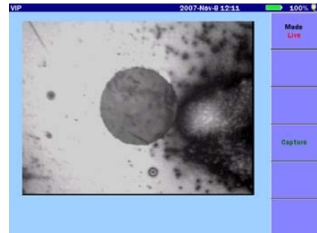
Dirty optical connectors can reduce system performance and often require costly troubleshooting to correct.
