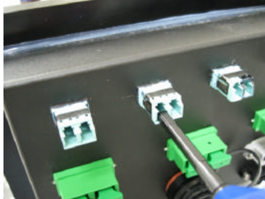
Figure 4. Cleaner with durability test apparatus
